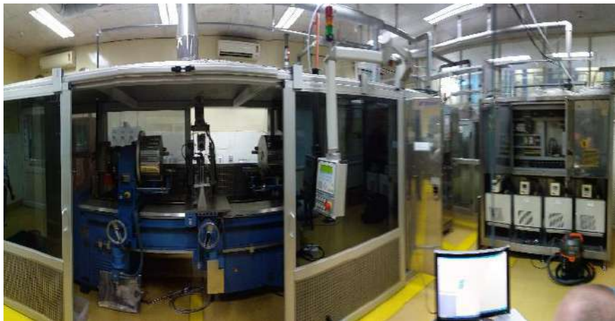
Fig. 7: MCVD System with high temperature vapor delivery unit for making laser fibers. (Nextrom, Finland)
