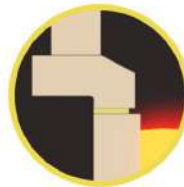
Jointing: Tuckstones and Sidewall
